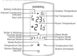
" \( '' \), " Temperature Set Buttons: Increasing or reducing the temperature while manual mode is active.
