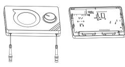
As shown in the picture above, press the screwdriver forward from the space shown, bend the tabs and separate the front cover. Insert 2 new AAA alkaline batteries in the battery housing with the correct battery direction. Replace both batteries at the same time. Then align the front part of your Room Thermostat to the back and squeeze it towards the back
