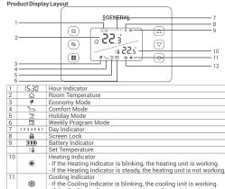
Note: During active use of the room thermostat, the symbols indicated by 3, 4, 5, 6, 10, 11 and 12 will not appear on the screen.
